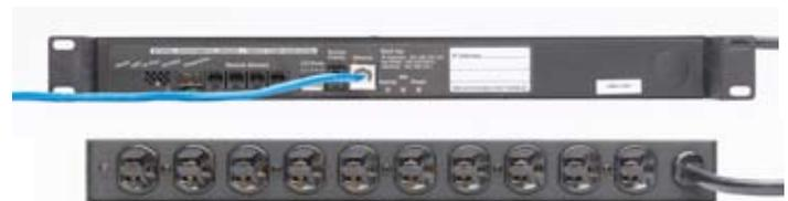
*No client software or installation CD is required. The user connects an Ethernet cable, sets the IP address and begins using the unit. An LCD constantly displays the sensor values.*
