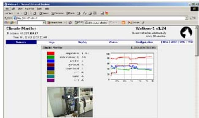
*A web page displays the current values with graphs showing trends. The web cam image is JPEG format. The data can be viewed on a PDA and cell phone. The unit is configured via the web page. Multiple alarm thresholds can be set with multiple e-mail alarm addresses.*
