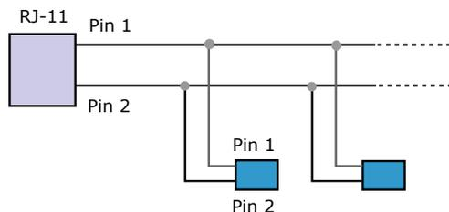
Multidrop wiring permits 16 temperature sensors to be added to any WeatherGoose Climate Monitor. The sensors are polarity sensitive. Each sensor is automatically discovered by the Weather Goose and can be given a friendly name.
