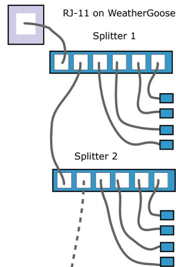
Telephone splitters can be used to add additional sensors up to the maximum of 16. Note that the temperature sensors are polarity sensitive. Splitters with a "crossover" wiring arrangement will not work. Telephone punch-down blocks can be used.
